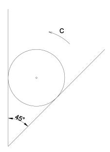
Assuming that friction is limiting at both the wall and the plane, show that the greatest couple, C, that will not rotate the cylinder is given by
