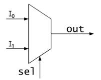
The company that you are working for requires to connect 4 devices  $(I_0 - I_3)$ , one at a time, to a single machine through the use of a 4-1 multiplexer.
