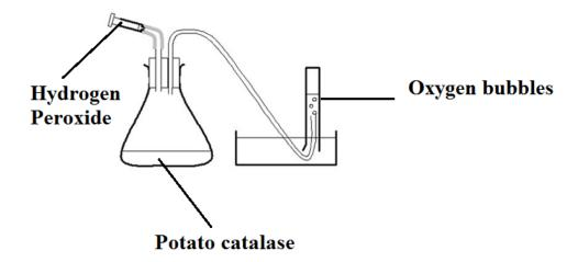
Figure 6.1: The apparatus used to investigate the effect of pH on enzyme-catalysed activity
