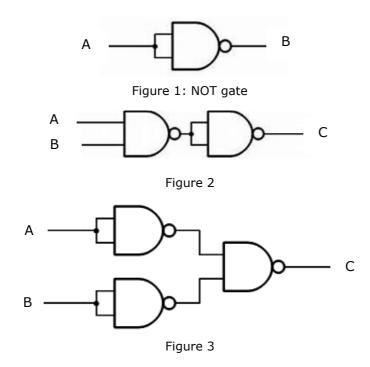
The function of the logic circuit in Figure 1 is that of a NOT gate (B = NOT A). By using truth tables, determine the function of the logic circuits in Figure 2 and Figure 3. (Hint: In cases where there is one input for a two-input gate, the same input should be used twice.)
