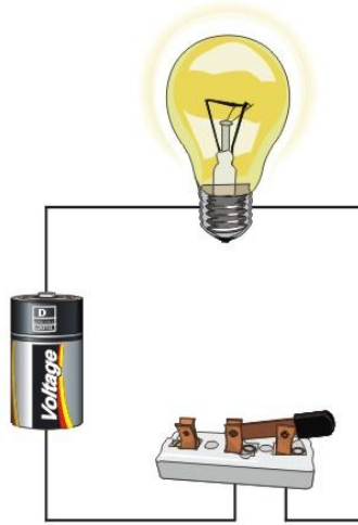
Figure 2- Light bulb circuit.
