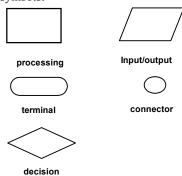
\* The use of structure diagrams and pseudo-code for describing an algorithm.
