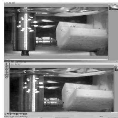
Figure 1: Nanoindentation of bone in liquid cell setup
