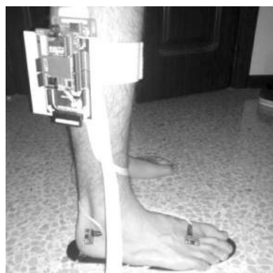
Fig 1 – The system to acquire and visualise foot posture and plantar pressure
