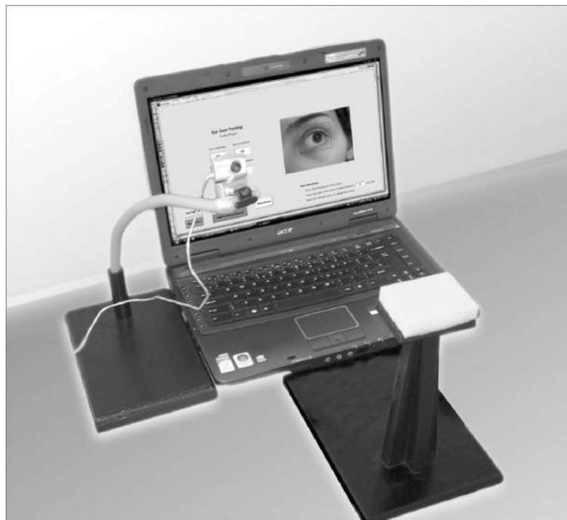
Low-cost eye-gaze tracking platform comprising an inexpensive webcam
