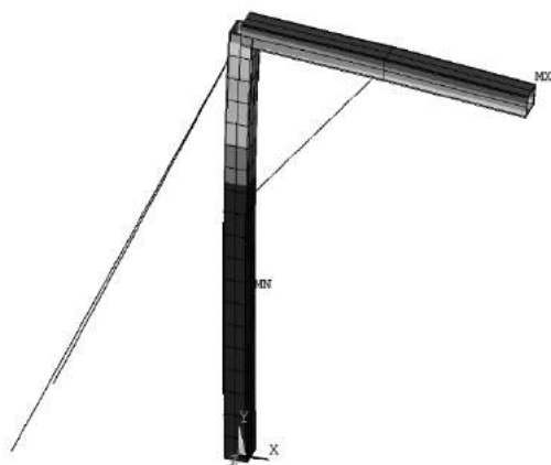
Figure 1: Finite element analysis to investigate deflections of main members
