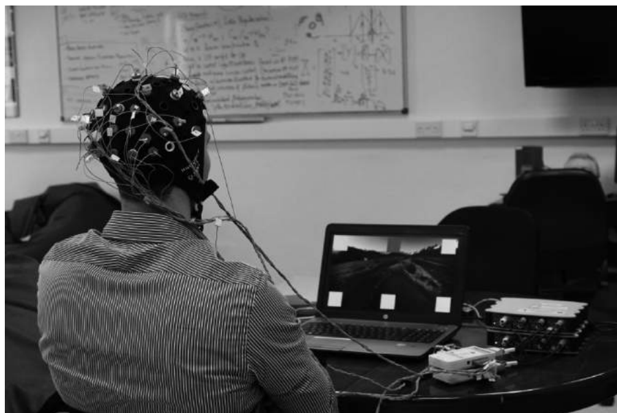
Brain controlled application based on steady-state visually evoked potentials (SSVEPs)
