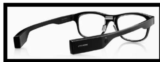
Typing using eye movements recorded through the Jins Meme EOG glasses
