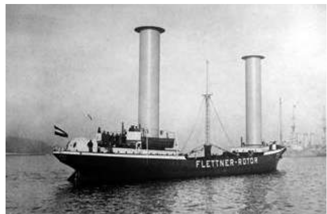
Figure 1: The first ever Flettner rotor, built in 1924
