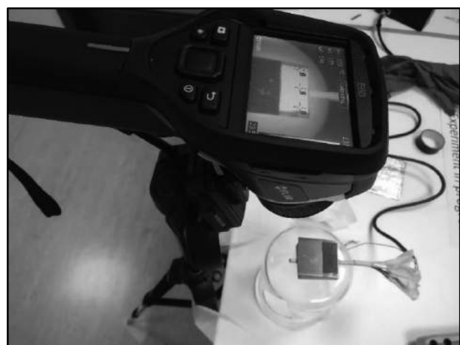
Figure 2: Thermal Imaging Setup using FLIR E60
