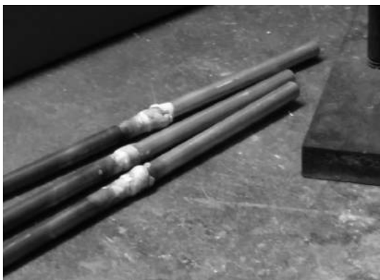
Figure 1: Pipe joints right after brazing
