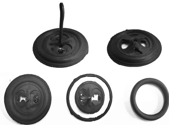
Figure 2: The demoulded parts were de-flashed using a blade and polished using a sand paper
