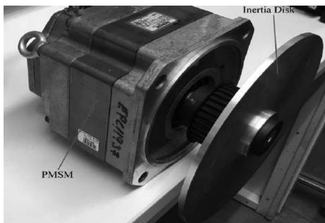
Figure 1: PMSM with inertia disk
