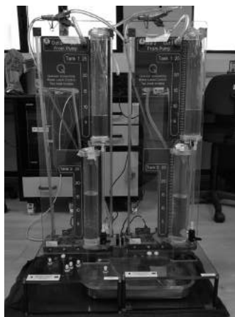
Figure 1: The Quadruple tank system (QTS)
