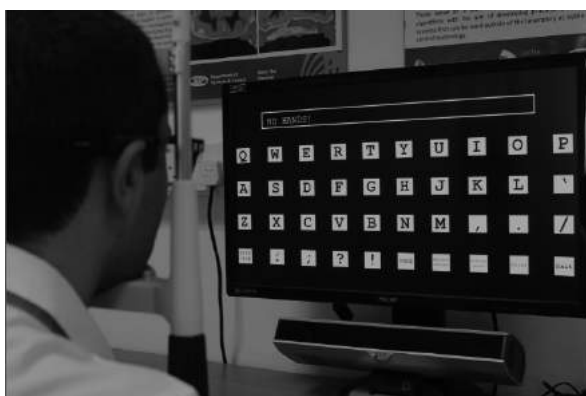
Typing using eye movements recorded through the Jins Meme EOG glasses
