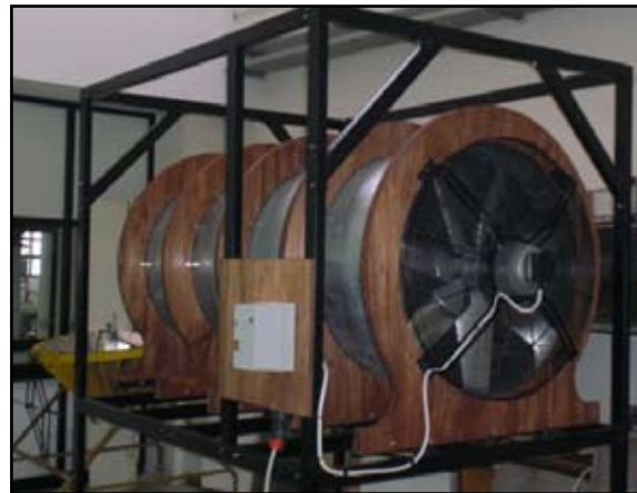
Figure 1: Low speed open jet wind tunnel
