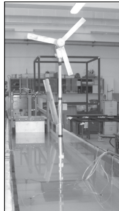
Figure 1: The model floating wind turbine that was constructed, and assembled in the wave tank.
