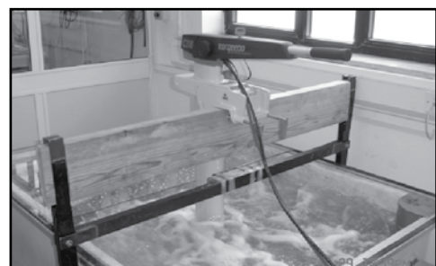
Figure 3 Motor in Test Tank
