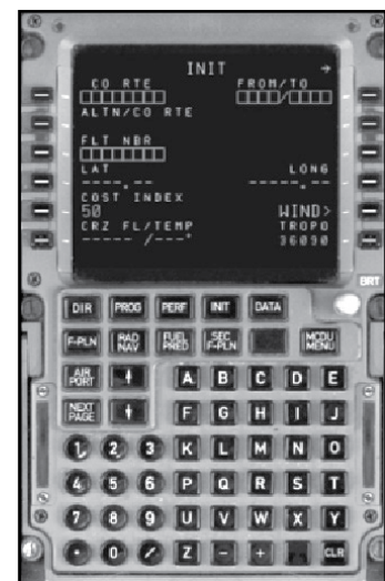
Figure 1: The developed MCDU simulator has an overlay image implemented on a touch screen, to make it look and feel realistic.
