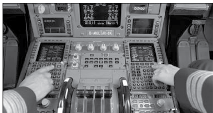
Figure 2: The MCDU is located on the central pedestal. It gives the crew immediate access to the flight handling functionalities.
