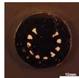
Figure3: Crevice Corrosion on ASTM F1586 (scale 10mm)
