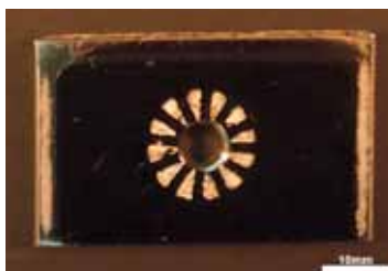
Figure1: Crevice Corrosion on AISI304 SS (scale 10mm)
