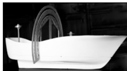
Figure 3: 1:15 fibre glass model adapted for the experiment
