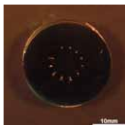
Figure2: Crevice Corrosion on AISI316 SS (scale 10mm)
