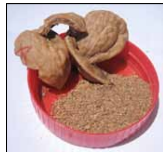
Figure 3: Ground walnut shells used as abrasive.
