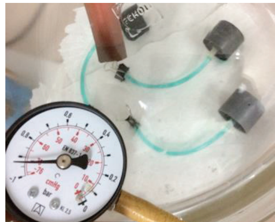
Figure 1: Toly's standard TM-71 Vacuum Test
