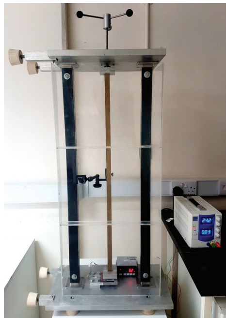
Figure 2: The Buckling Apparatus Set-up
