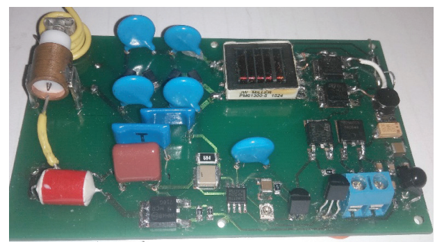
Figure 2: Prototype PCB with PPT and power supply
