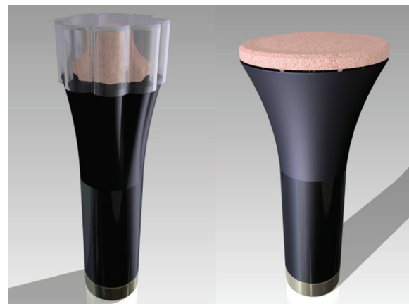
Figure 2: Rendered images of the PAMeIA in the curved and flat states
