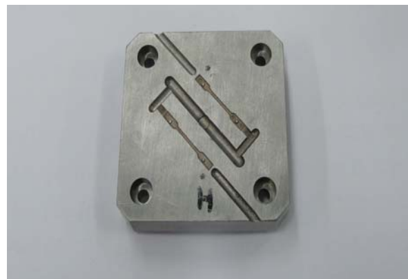
Figure 2: A finished mould insert
