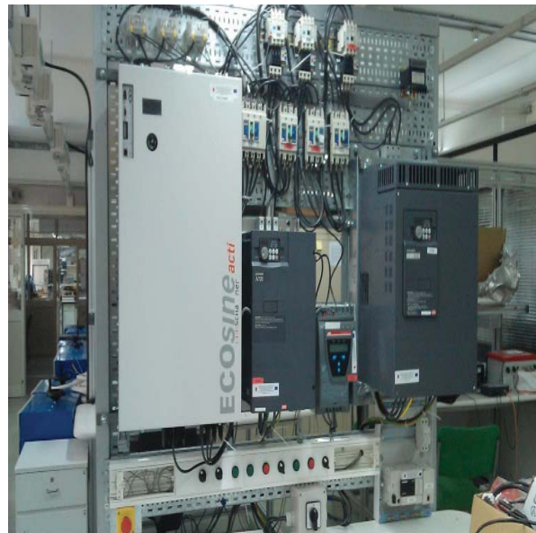
Figure 1: Active Filter Setup
