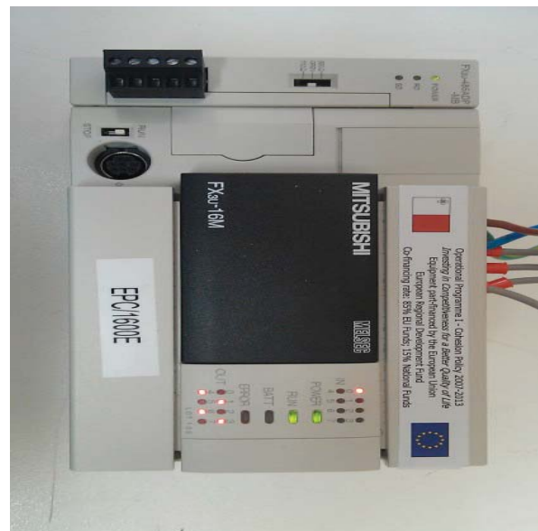
Figure 2: Programmable Logic Controller
