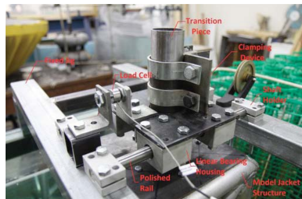
Figure 2 – Model Jacket Structure Mounted in Wave Tank
