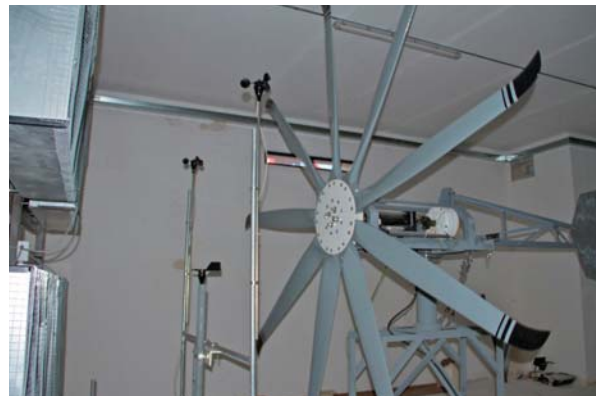
Figure 1 - Wind Turbine with Wind Monitoring Sensors and Fans
