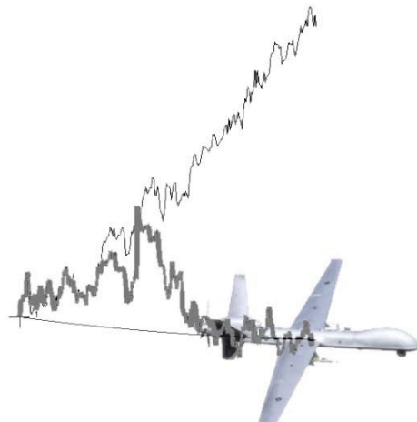
Figure 2: Results with dead reckoning errors (narrow line) and errors after correction (bold line)
