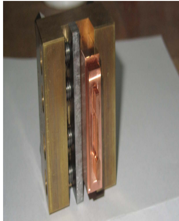
Figure 1: Micro tensile specimen copper electrode
