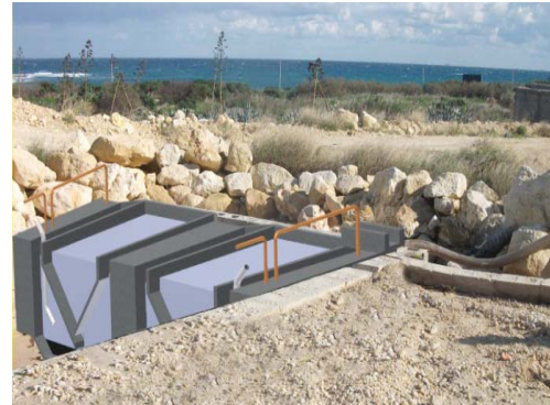
Figure 1: Photomontage of proposed Imhoff Tank (cross-sectioned)
