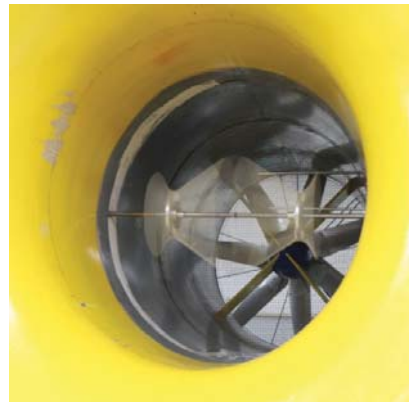
Figure 1: The VAWT model operating in the wind tunnel
