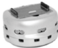
Figure 2: The Khepera III Robot with Korebot II Microcontroller
