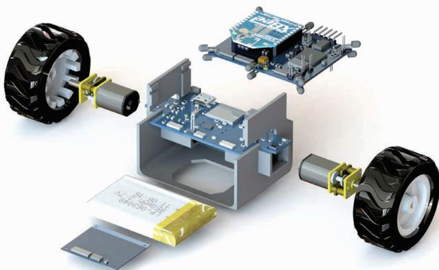
Figure 1: Exploded View of the Robotic Platform
