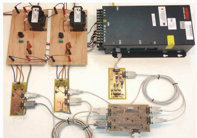
Figure 2: The Constructed 24V DC Microgrid
