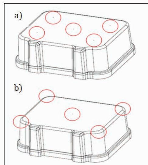
Figure 1: a) Current mould used at Playmobil Malta Ltd. b) New mould designed
