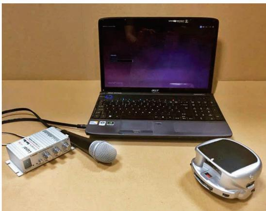
Figure 1: The hardware and Khepera III mobile
