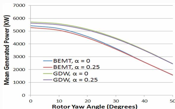
Figure 2: Graph of Mean Generated Power (KW) Against Rotor Yaw Angle (Degrees) for the TLP FOWT.  $H_w = 1.5$  m,  $T_w = 5.5$  s
