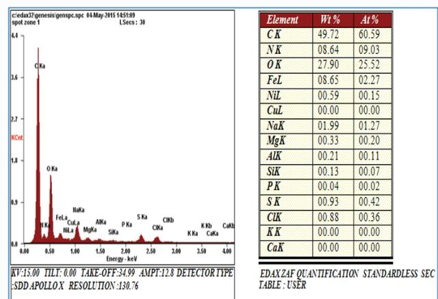
Figure 2: EDS Analysis of Membrane Cleaned with the standard WSC procedure, at 200X
