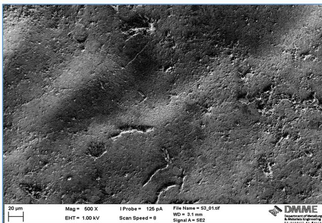
Figure 1: Scanning Electron Micrograph of a Membrane Cleaned with the standard WSC cleaning procedure at 500X
