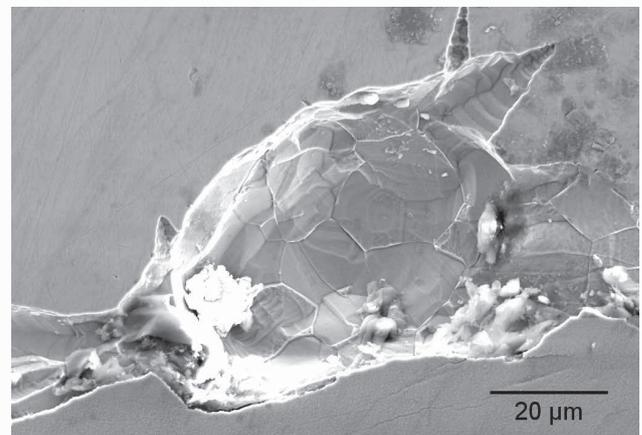
Figure 1: Pitting present in CrN coatings following tribocorrosion testing in Ringer's Solution against an inert alumina ball
