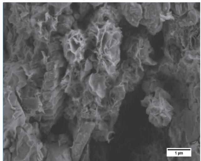
Figure 1: Electron micrograph of the deposited calcium phosphate rich mineral onto clean limestone
