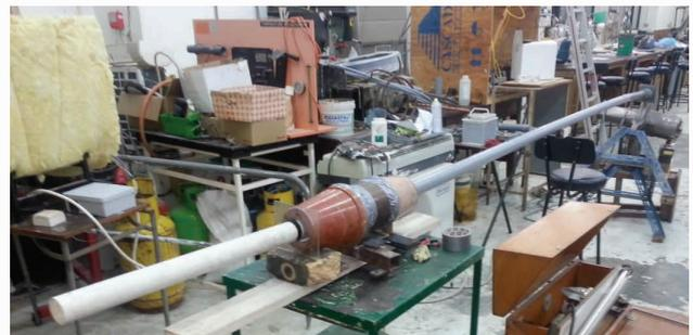
Figure 2: Air Flow Setup for DPF Section
