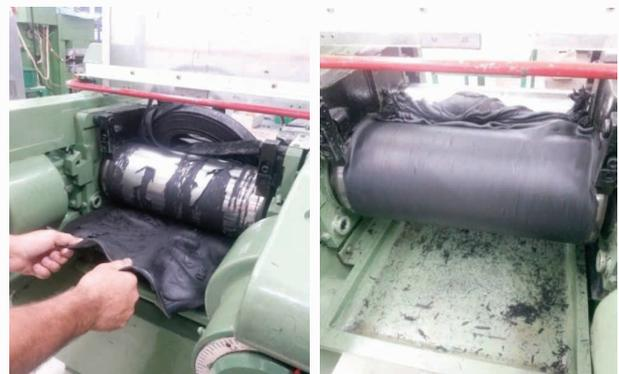
Figure 1: Initial raw material feeding in the calendering machine
