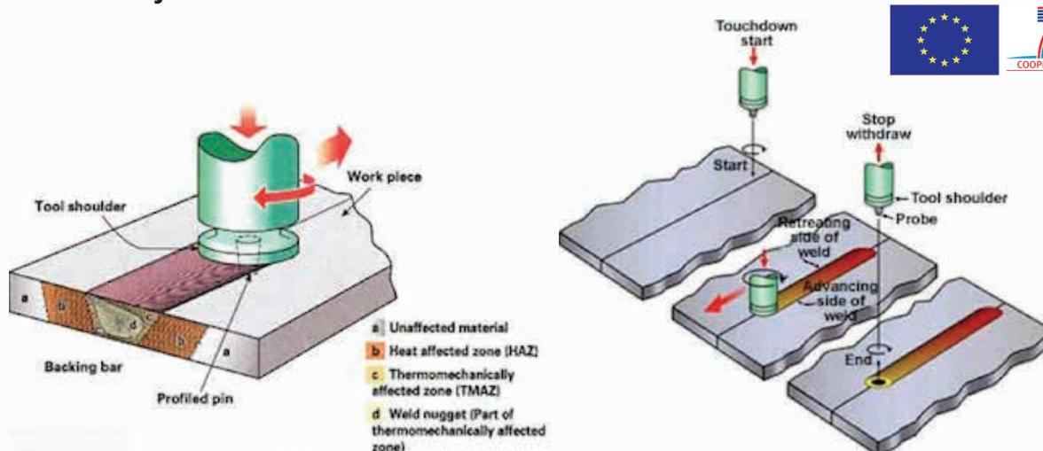
*Generic principle of friction stir welding (Courtesy of TWI Ltd)*
