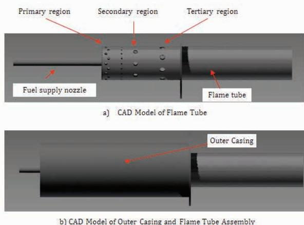
Figure 1: CAD Model of Combustion Chamber Assembly
