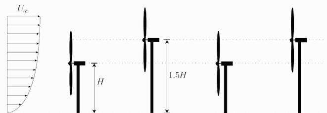
Figure 2: Staggered height configuration
