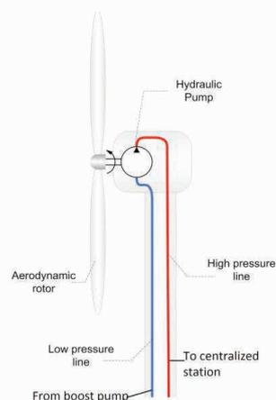
Figure 2: Overall System Schematic [1]
