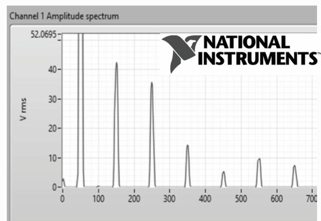
Figure 2: LabVIEW GUI Amplitude Spectrum
