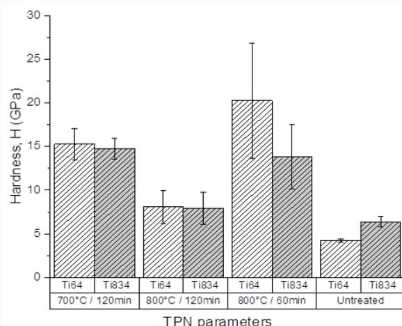
Figure 2: Hardness values for untreated and TPN treated Ti64 and Ti834
