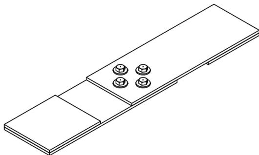
Figure 1: Four bolted lap connection
