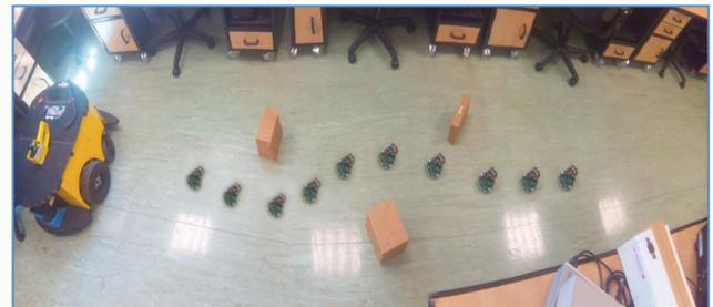
Figure 1: Typical path taken by the robot when approaching the target using DWA
