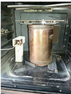
Figure 1: DPF Section in the Furnace
