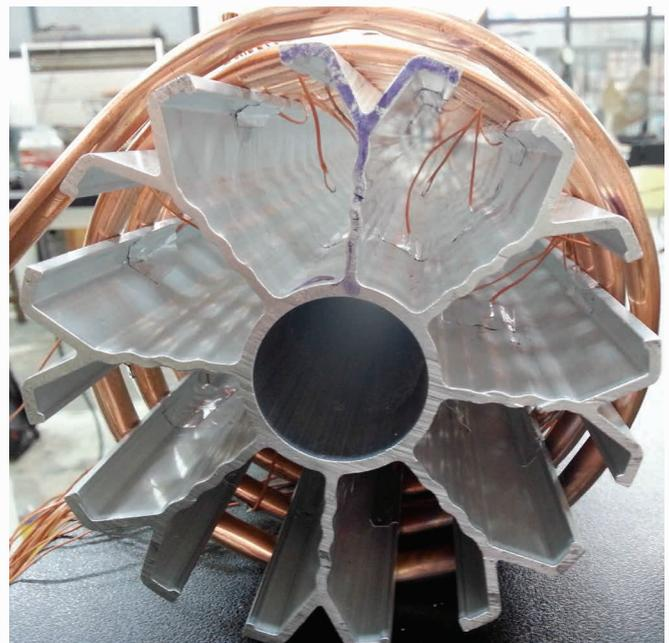
Figure 1: The aluminium core with thermocouples attached, wound with copper tube
