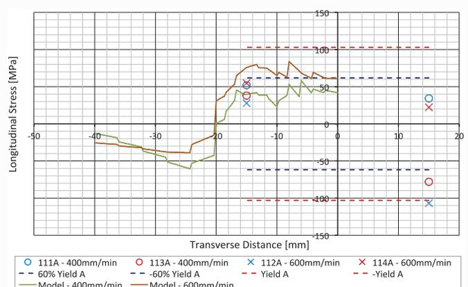
Figure 2: Longitudinal Stress (MPa) vs. transverse distance (mm) for Al 1050-H14, welded to ultra low carbon steel; experimental values by [2]
