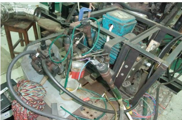
Figure 1: Injector flow test bench
