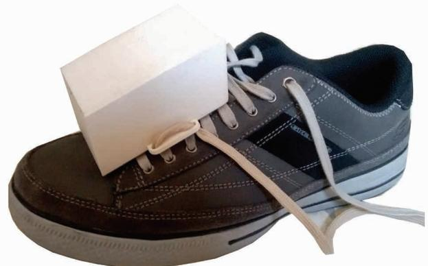
Figure 2: 3-D printed PLA casing mounted on shoe
