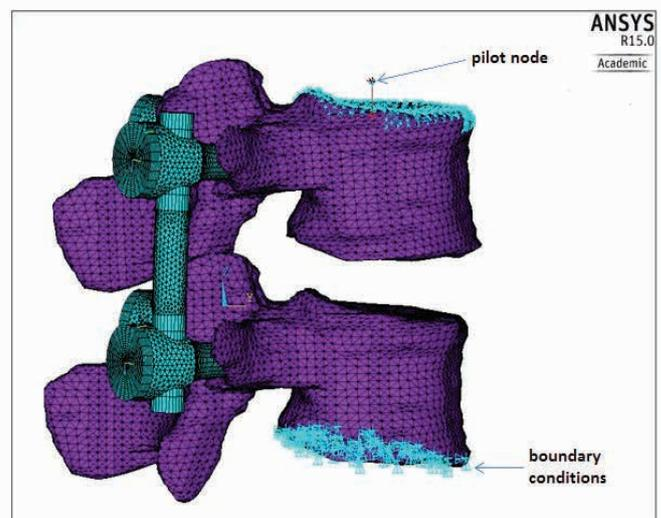
Figure 1: Loads and boundary conditions imposed on the meshed assembly
