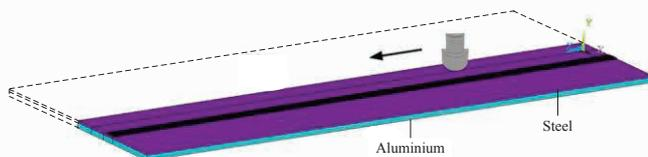
Figure 1: Half the geometry of the model. FSW tool advancing in the direction of the arrow
