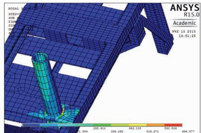
Figure 1: Stresses Experienced by the Nacelle Structure and Yaw Shaft during Normal Operation (Bottom View)
