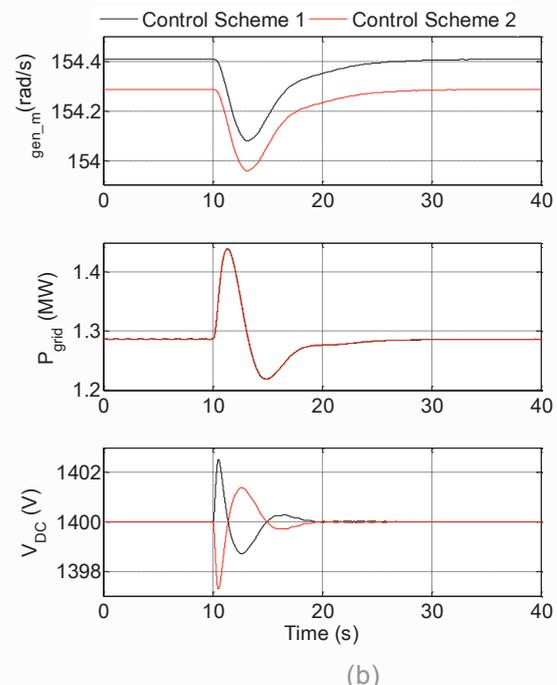
Figure 1: PMSG based FRC WT model (a) and WT frequency event response (b)
