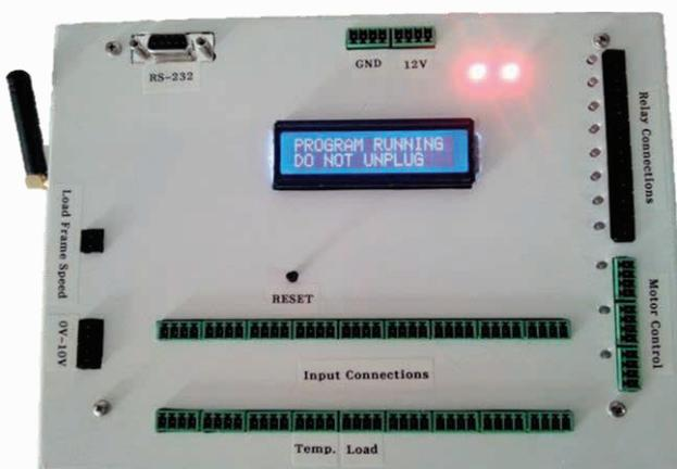
Figure 1: Data Acquisition and Control Board
