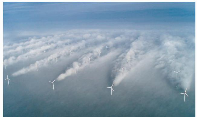
Figure 1: Wind turbine wake [1]
