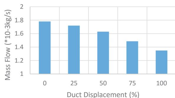
Figure 2: Mass flow rate variation in the models with different duct misalignments
