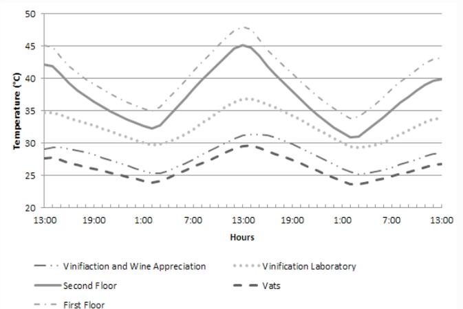
Figure 2: Temperature in different zones
