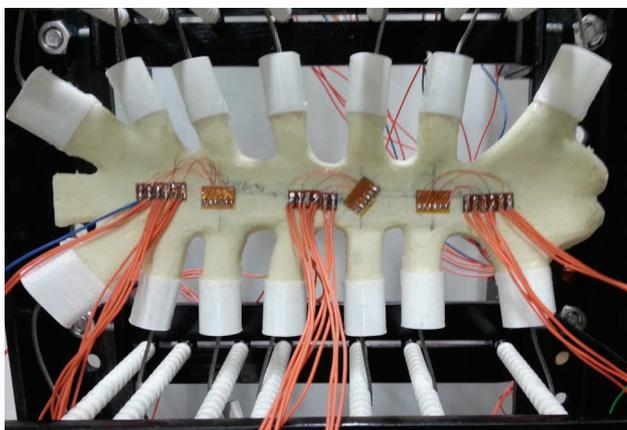
Figure 1: Sternum model mounted in testing frame
