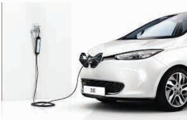
Figure 1: Residential Mode 2 Charging Electric Vehicle [3]
