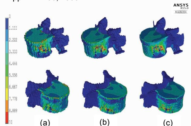
Figure 2: von Mises stress distribution on application of a 2000 N force on the vertebral body of the 3x3, (a) Heterogeneous; (b) Alternative Equation; (c) Homogeneous model. Scale is given
