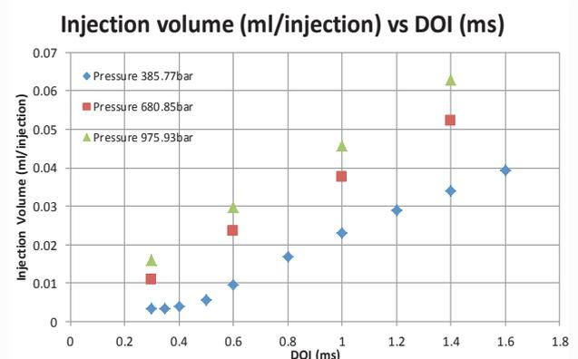
Figure 2: Injection volumes at different pressures
