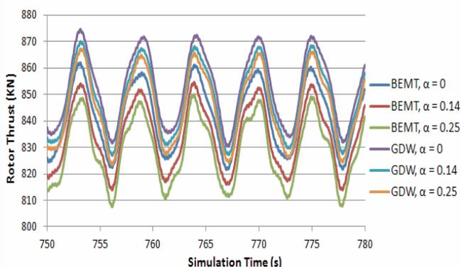
Figure 1: Graph of Rotor Axial Thrust (KN) Against Simulation Time (s) for the TLP FOWT.  $H_w = 1.5$  m,  $T_w = 5.5$  s
