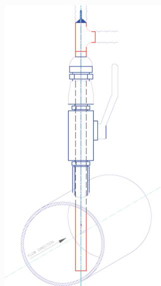
Figure 2: Accutube inserted in Test Pipe
