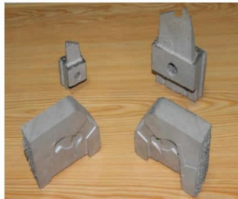
Figure 1: Two inserts and sliders fabricated using SLM
