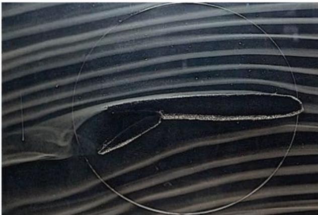
Figure 1: Experimental Flow Visualisation of a NACA 2412 aerofoil with a Split Flap at 0°
