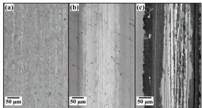
Figure 1: SEM image showing corrosion-wear scar morphology on (a) 316 LVM stainless steel, (b) Cr-C coating, (c) Zr-C coating, following tribocorrosion under 1 N load in Ringer's solution.
