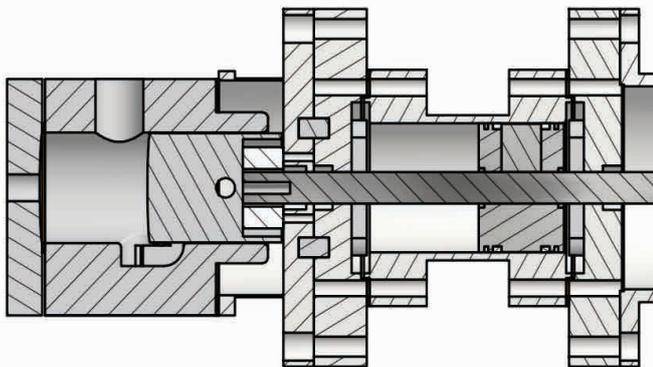
Figure 1: Left Section View of the Free-Piston Engine
