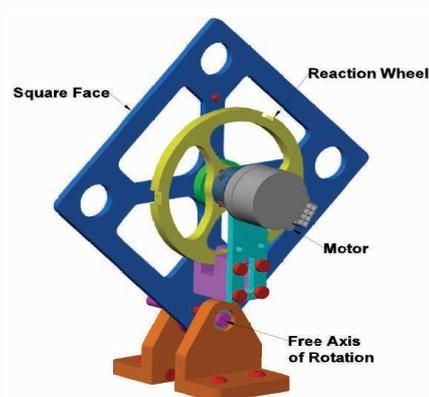
Figure 1: CAD Drawing of the Mechanical Setup
