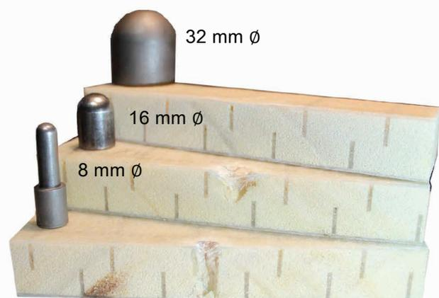
Figure 2: Sectioned sandwich specimen illustrating indentation
