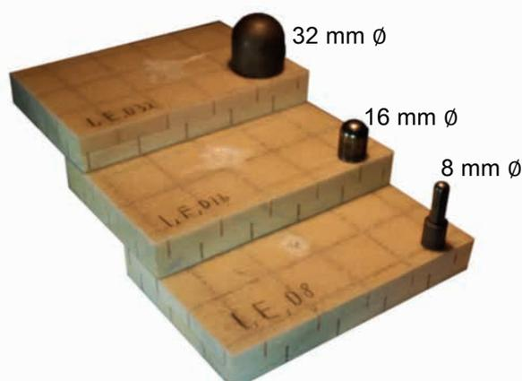
Figure 1: Sandwich specimen showing surface damage
