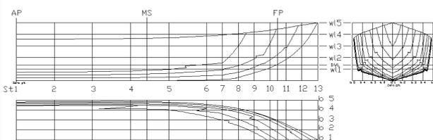
Figure 1: Lines plan of the new hull design
