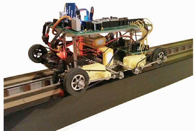
Figure 2: Vehicle Model in Magnetic Levitation Mode
