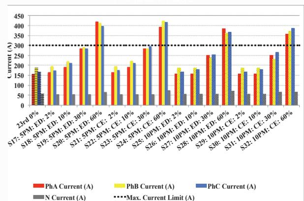
Figure 2: Maximum Phase and Neutral Current from Simulated Scenarios
