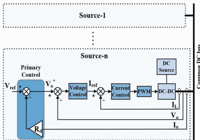
Figure 1: Primary Control of DC Microgrids
