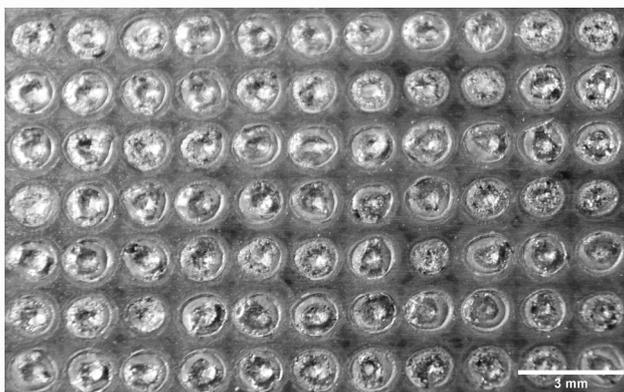
Figure 1: Pattern of laser spots on the surface of ADI
