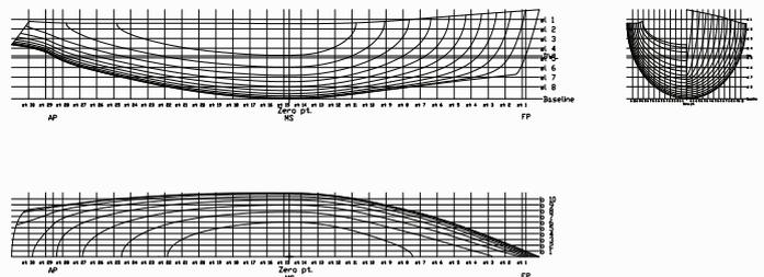
Figure 1: Lines plan for the designed hull
