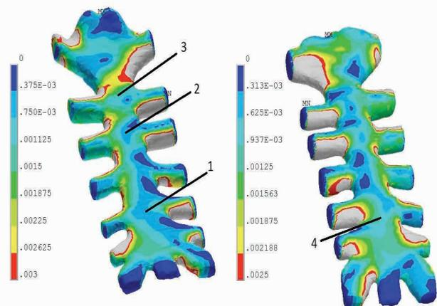
Figure 2: Finite element model with labelled rosette locations: left – front, right - Back
