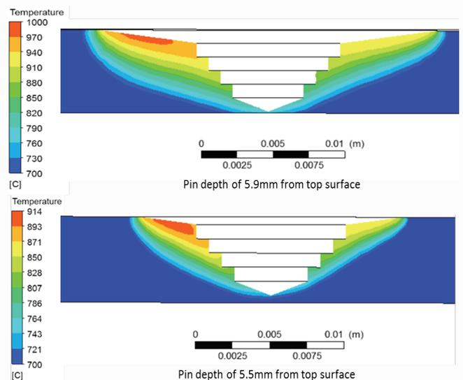
Figure 1: Effect of pin penetration depth
