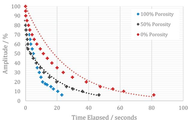
Figure 1: Decaying Time-Response of Initial Signal
