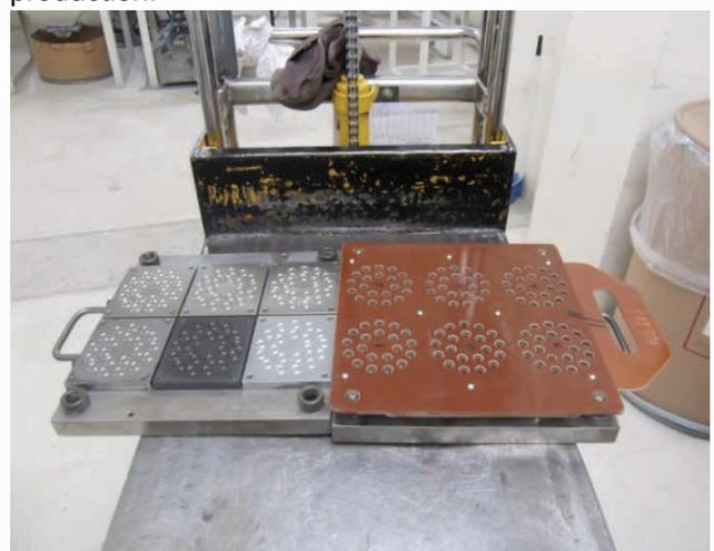
Figure 1: The segmented mould used in the in-field testing
