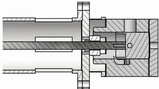
Figure 2: Right Section View of the Free-Piston
