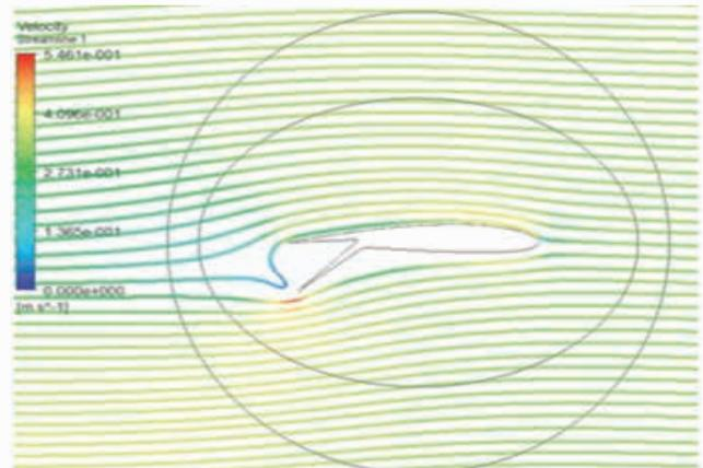
Figure 2: Computational Flow Visualisation of a NACA 2412 aerofoil with a Split Flap at 0°
