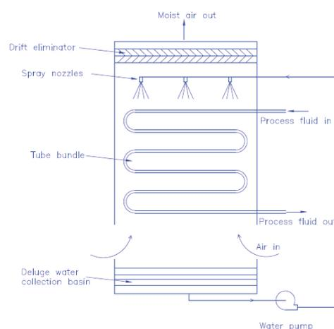
Figure 1: Closed Circuit Evaporative Cooler
