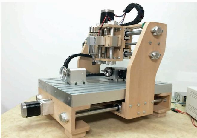
Figure 1: Final Designed 4-Axis CNC Milling Machine
