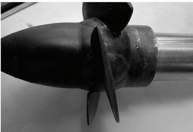
Figure 1: Model of Kaplan Turbine
