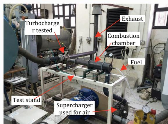
Figure 2: Test Stand Constructed
