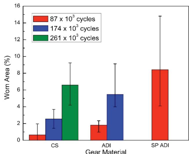
Figure 2: Percentage worn area of gear teeth for the different tested materials.
