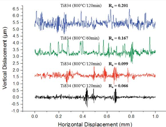
Figure 1:  $R_a$  values for untreated and TPN treated Ti834
