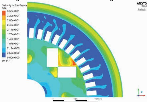
Figure 1: Velocity contour plot through the centre of the radial duct of the in-line model
