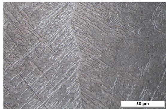
Figure 2: Typical acicular microstructure within prior-β grains
