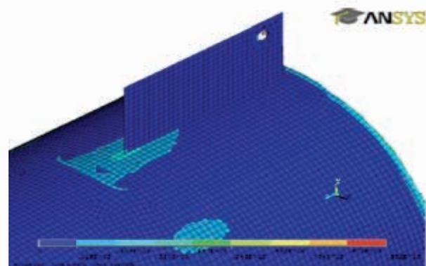
Figure 1: FE model of main cylindrical shell and towlug
