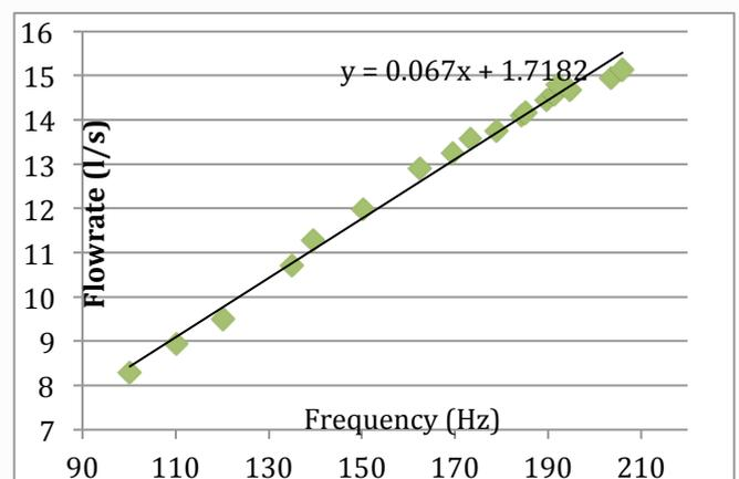
Figure 2: Graph of Flowrate (l/s) vs Frequency (Hz)
