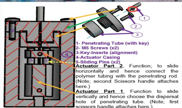
Figure 1: Top - Manufactured prototype with detail on dispersal Canals. Bottom – Section view of actuator Casing with labelled 'hidden' parts.
