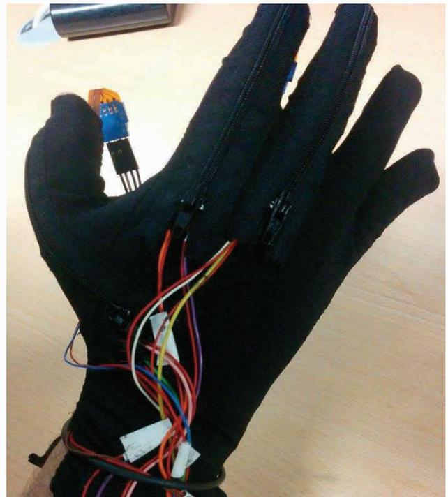
Figure 1: Glove master device
