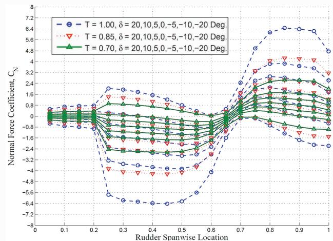
Figure 2: Force coefficient,  $C_N$  across the rudder span for  $X/D = 0.35$ .
