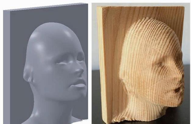
Figure 2: Part CAD Model (left) Machined Result (right)
