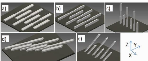
Figure 1: Different lay orientations studied – a) XY b) ZX c) ZY d) 30° to XY plane e) 60° to XY plane
