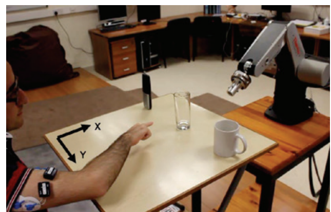
Figure 1: Controlling the wrist position of a robotic arm using muscle activity recorded from the human subject
