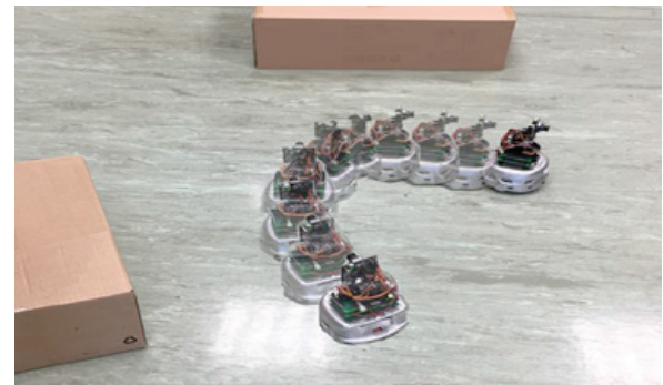
Figure 1: The trajectory followed when the Khepera III mobile robot encountered some obstacles during a search operation
