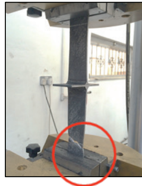
Figure 1: Cruciform specimen after failure at the plate Table 1: Ultimate load results (FEA, Exp., EN1993)
