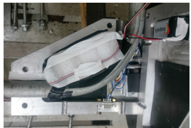
Figure 2: Anemometer Circuit inside Fixture
