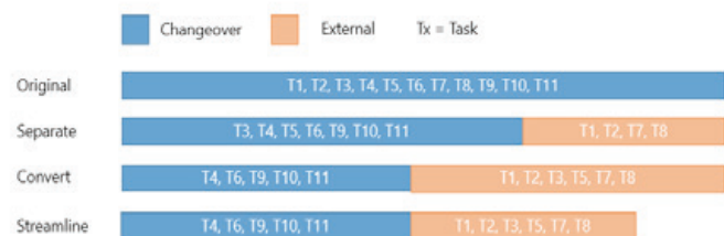
Figure 2: Applying the SMED Methodology to the Case Study Changeover
