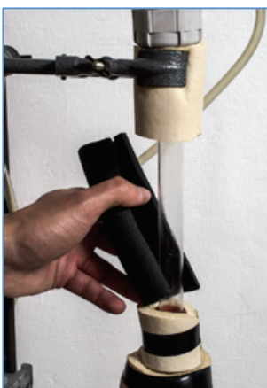
Figure 1: Exposing glass adiabatic section
