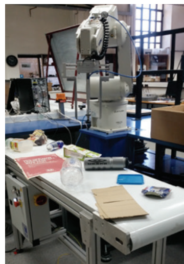
Figure 2: The various materials having different shapes and sizes handled by the gripper
