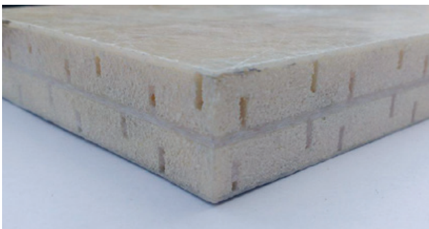
Figure 1: Multi-Layer Sandwich Panel
