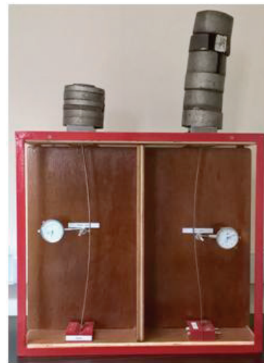
Figure 1: Testing the buckling of struts apparatus
