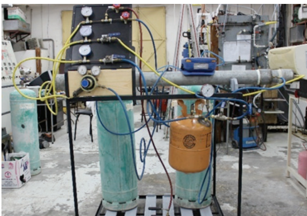
Figure 1: System for Biogas Purification
