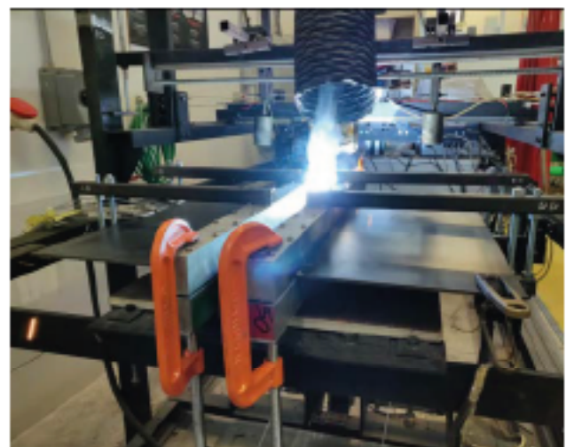
Figure 1: Automatic MIG Welding in process
