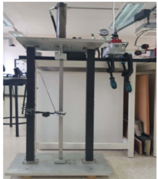
Figure 1: The buckling experiment set-up
